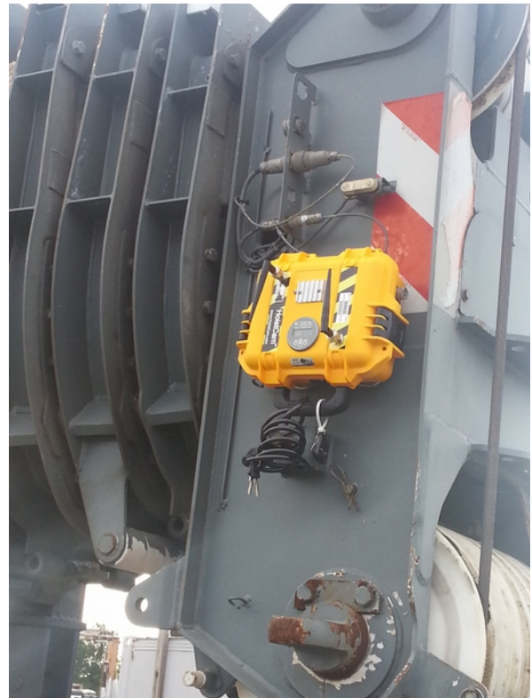
Wireless Repeater (RPT103) Attached to Boom Tip with HoistCam
