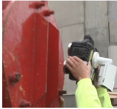
Install HoistCam on Block In a Minute with Magnets
