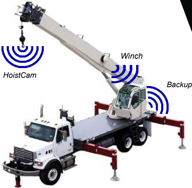
Split Screen Display with Wireless HoistCam and Wired Cameras
